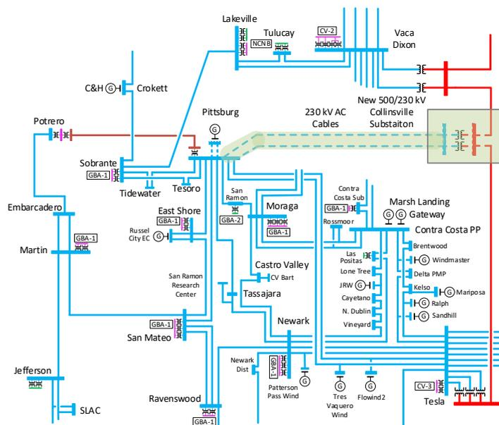
The ISO estimates that the proposed project will approximately cost \$475 to \$675 million. The project is to be in-service no later than June of 2028. Figure G2-1 provides a schematic diagram of interconnection to the Pittsburg 230 kV substation.
