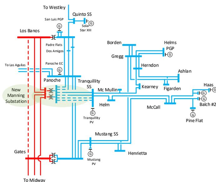
The ISO estimates that the proposed project will approximately cost \$325 to \$485 million. The project is to be in-service no later than June of 2028. Figure G1-2 provides a schematic diagram of the interconnection to Tranquillity 230 kV substation and an approximate area for the location of the Manning substation.
