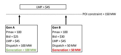
**Total Generation:** Gen A + Gen B > 150 MW > POI constraint limit
