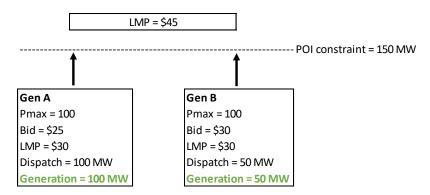
Total Generation: Gen A + Gen B = 100 MW + 50 MW = 150 MW = POI constraint limit
