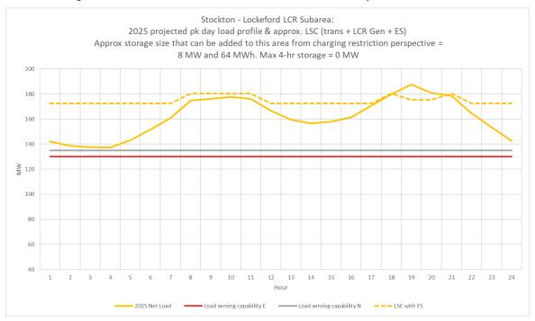
Figure 3.3-26 Lockeford LCR Sub-area 2025 Forecast Hourly Profiles
