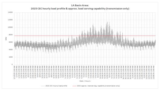
Figure 3.3-89 Western LA Basin LCR Sub-area 2025 Load Shape and Estimated Maximum Energy Storage Capacity and Energy Based on Charging Capability Under Critical Contingency
