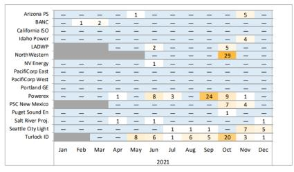
Figure 3.13 Frequency of downward flexibility test failures by month and area (15-minute intervals)
