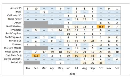
Figure 3.11 Frequency of upward flexibility test failures by month and area (15-minute intervals)
